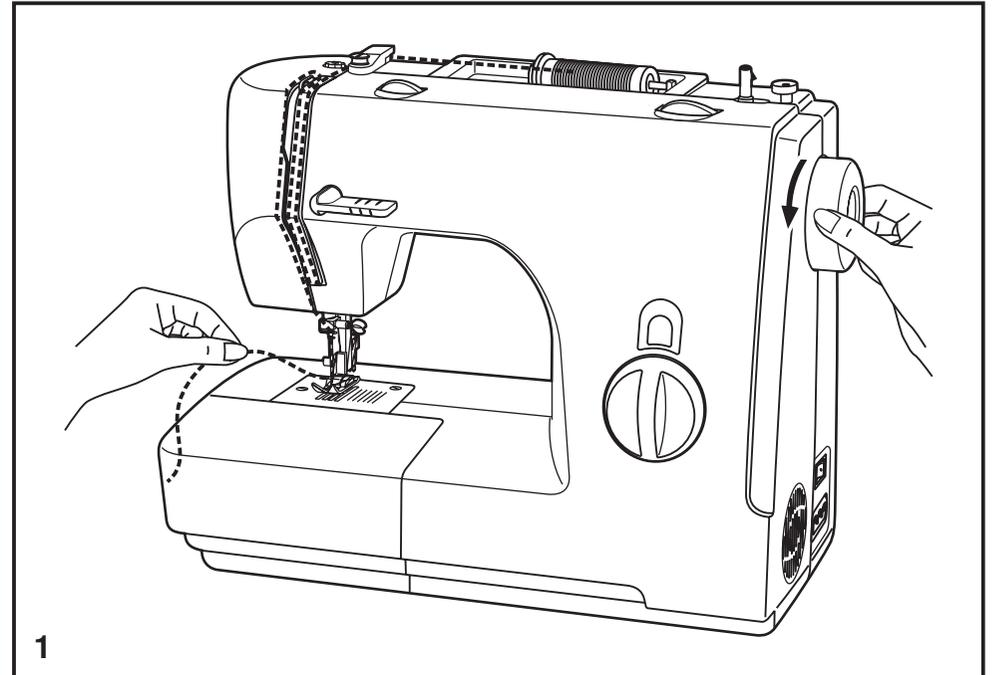
Gently pull on the upper thread to bring the bobbin thread up through the needle plate hole (2).
